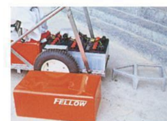
Stable Batteries Stand Allow Convenient Exchange of Recharged Batteries
